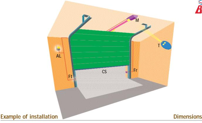
M operator EOS (P915140 00001) with SCE control board, and incorporated rolling-code receiver with 63 codes T double-channel rolling-code transmitter, Mitto 2 (D111453) Ft-Fr Pair of photocells, Cellula 130 (P111273) AL blinker Lampo 24V (D113638 00005) with antenna AEL 433 (D113632) CS Safety edge
