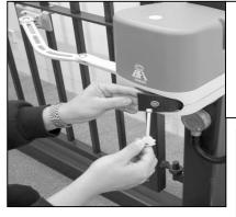
**BFT 'VIRGO' Articulated Arm.** Key release is within black pull handle at front of motor. Rotate clockwise to unlock and pull black handle. Rotate anti-clockwise to re-instate.
