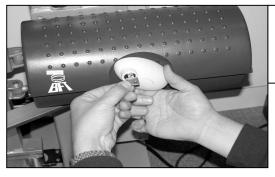
**BFT 'IGEA' Articulated Arm.** Turn the key in the lock and rotate the coloured plastic knob on the front of the motor to release the gate. Reverse the process when power is re-instated.
