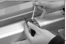
**BFT 'ORO' Hydraulic Ram** Key release is on top of motor 10" from the gate post end. Rotate triangular keyway anti-clockwise to release and open gate v.slowly. Reverse process to re-instate.
